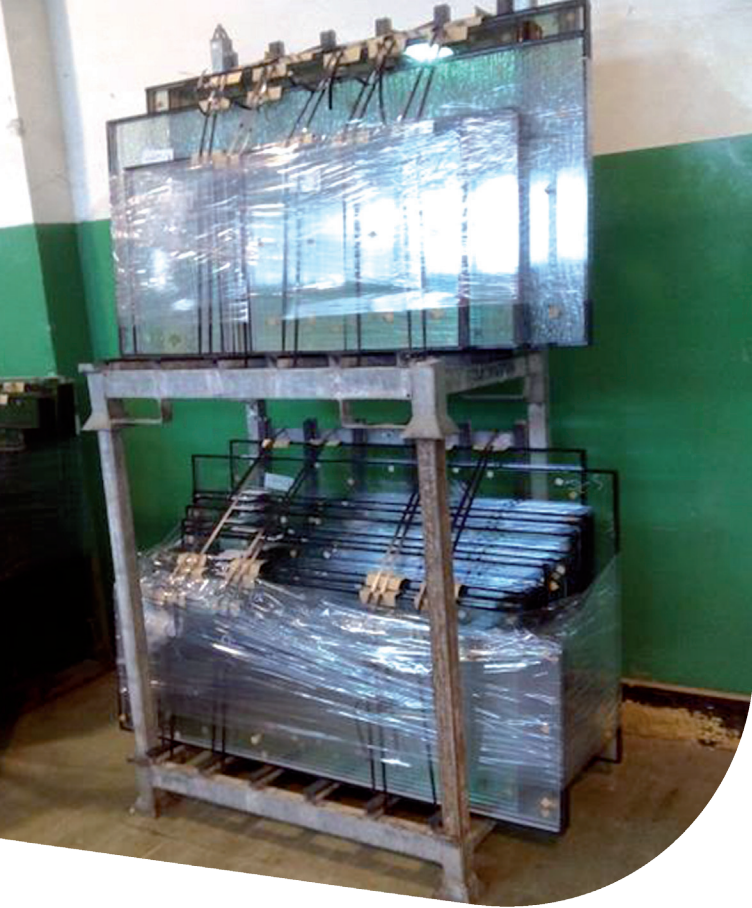
Fig. 25. L-type metal rack, stacked.
