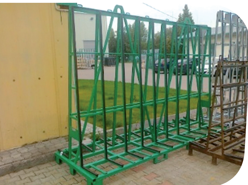
Fig. 24. MEGA/GIGA type metal rack.
