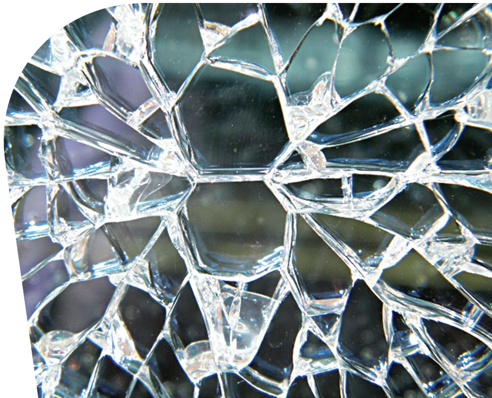
Fig. 10. View of the toughened glass fracture pattern in which a spontaneous breakage could occur due to NiS inclusion.
