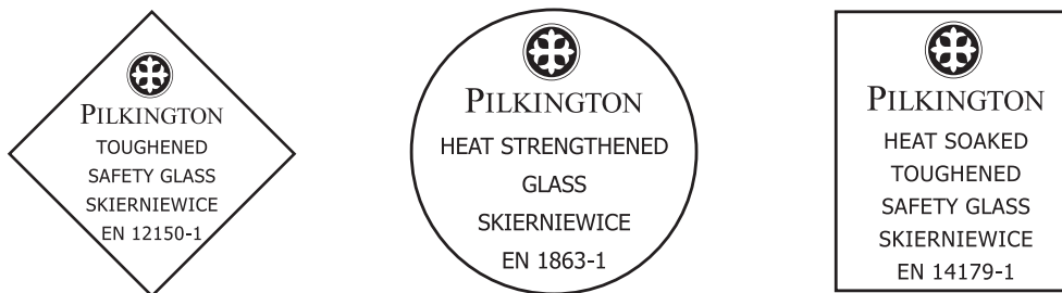
Fig. 3. Examples of permanent marking of toughened glass sheets, heat strengthened glass sheets and toughened and heat soaked glass sheets.
