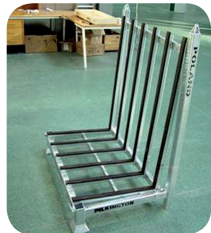
Fig. 23. L-type metal rack, stacked.
