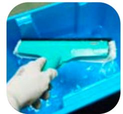
Hand window cleaner with a soft material cover (e.g. microfiber cloth) or soft cloth and rubber squeegee should be used as washing equipment. A large amount of water is necessary for glass cleaning as water is an universal neutral solvent for most of dirt.
