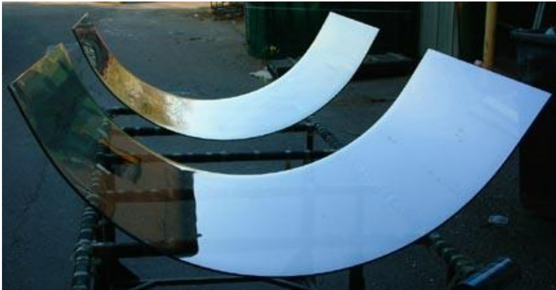
Successful Bending of 6 mm (1/4") Pilkington Eclipse Advantage ™ Clear
