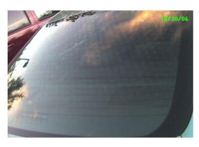
Typical dot quench pattern seen in a tempered Mercedes automotive back window when incoming light is reflected from a blue, or partly cloudy, sky. Notice the sun is not directly shining on the glass.
