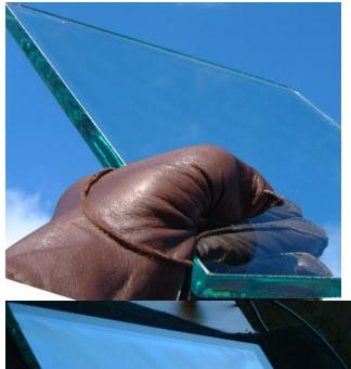
A 12inch square of 12 mm thick tempered glass can show its quench pattern to the naked eye, with no Polaroid filters, when viewed at appropriate angles on a blue sky day.
