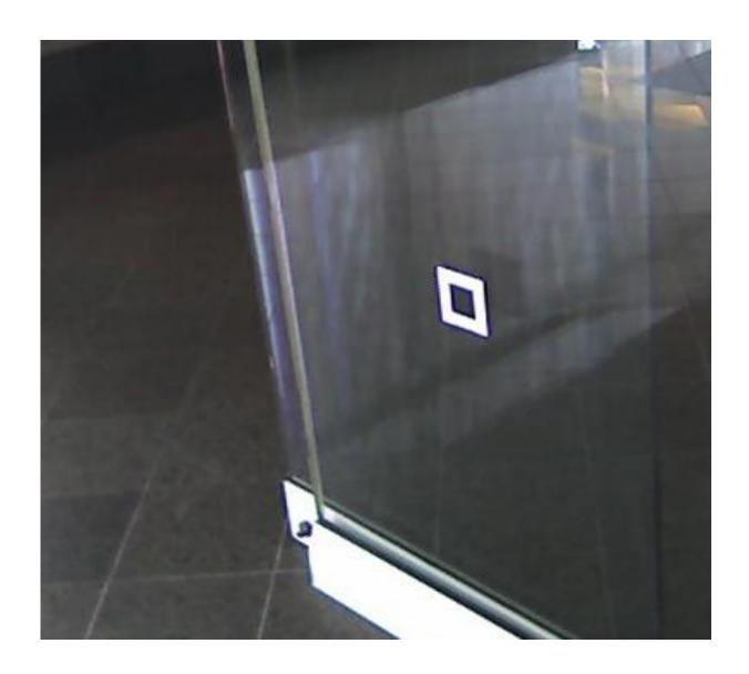
These 2 lights of 12 mm tempered glass in a sliding door at the Pittsburgh airport Hyatt hotel entrance, shown open with one light behind the other, display a strong quench pattern to the naked eye (no Polaroid filter). The incoming light (from lower left) is polarized by reflection off the polished stone floor; further reflections, again at Brewster's angle off the glass, add to the constructive/destructive interference effects.
