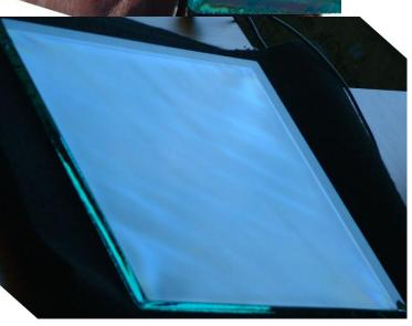
The same 12 inch square of 12 mm tempered glass much more readily shows the quench pattern under the same lighting and viewing conditions when viewed in reflection, with the transmitted image subdued by placing the glass on black velvet.
