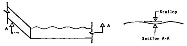
4. **Shell or Flake Chip** - This is a chip at a glass edge, usually smooth, having the appearance of a shell. Flake chips are generally more pronounced as glass thickness increases.
