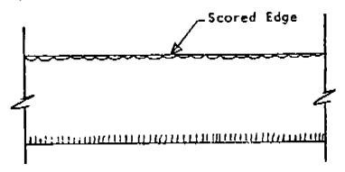
b. **Feather or Fishbone** - A group of dagger-like cracks that form in a slightly curved manner across the face of the glass as shown below:
