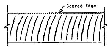
c. **Shark Teeth** - Dagger-like cracks starting at the scored edge and usually wide at the glass surface and pointed at some distance away from the surface as shown below:
