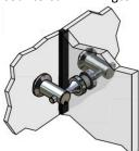
2. Countersunk Pilkington Planar™ 902 bolt with Nexus Casting
