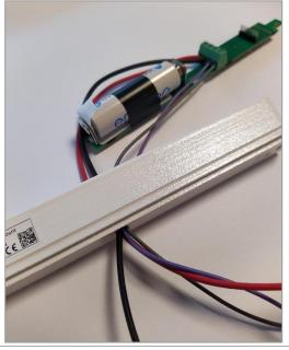
2. On the circuit board there is room to connect four (4) cables. (+) and (–) from glass and solar panel respectively. Cables have the following colors:
