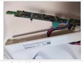
6. Test the connections by pressing the blue button on the circuit board.
