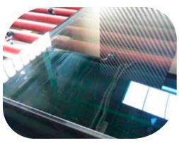
The results of glass cleaning with the use of steel blade – visible surface damages.
