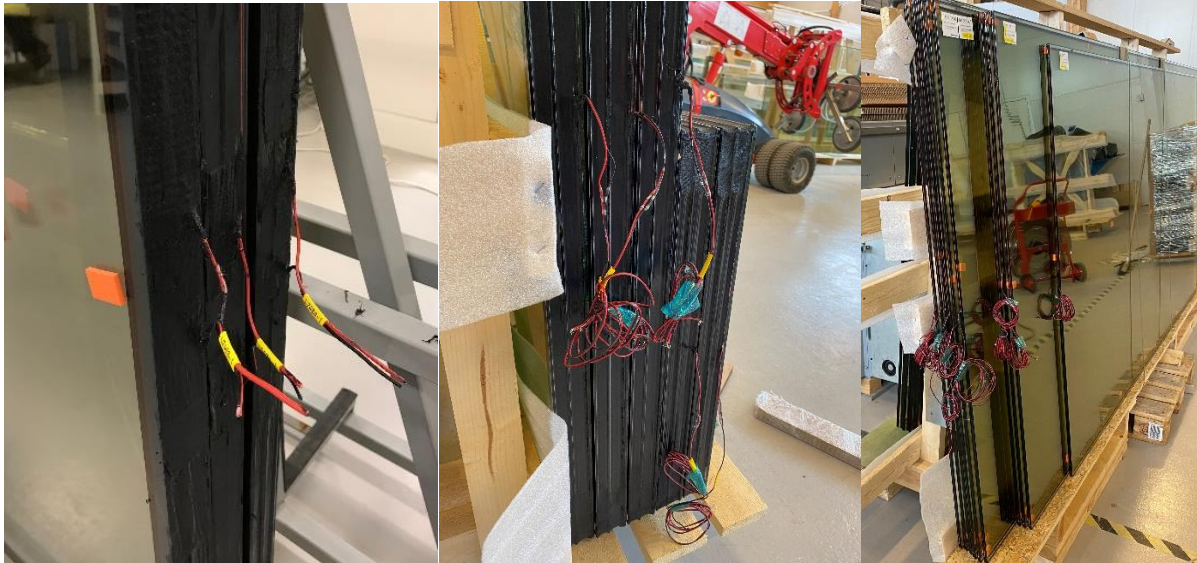
Figure 5. Example cable outlet ConverLight Dynamic; Left: Insulating glass short free-hanging cable outlet, where ID number is on yellow cable marking; Middle: Insulating glass longer coiled cable outlet, where ID number is on yellow cable marking; Right: Glass laminate with longer coiled cable outlet, where ID number is on yellow cable marking in a separate bag.
