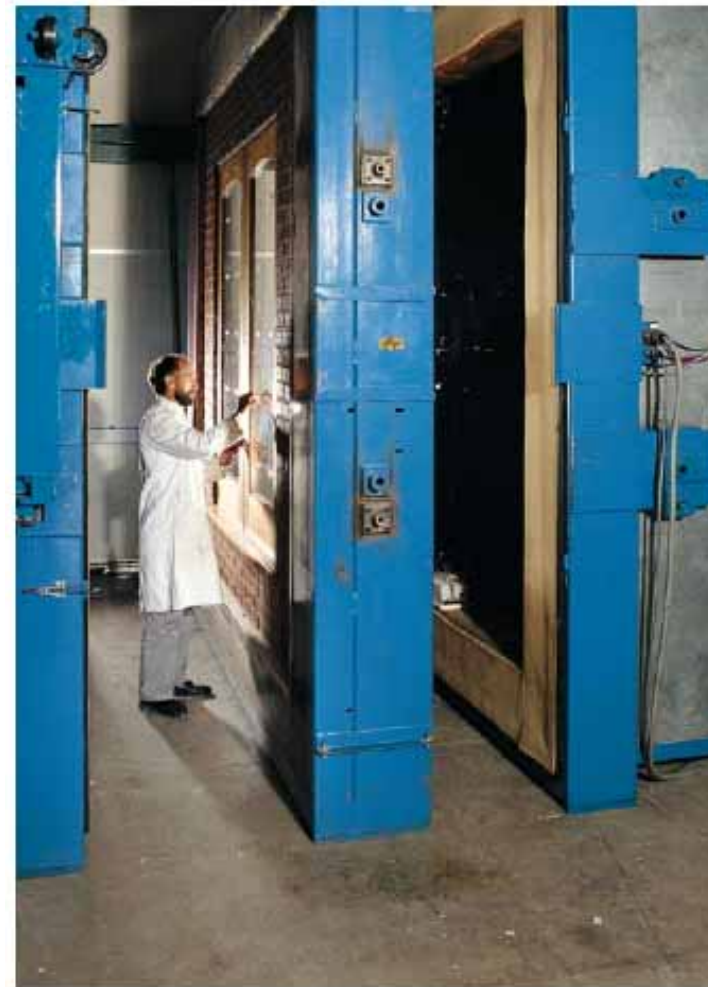
Hot Box apparatus, Pilkington United Kingdom Limited
