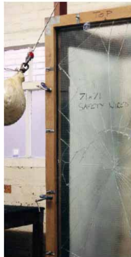
Pilkington Pyroshield Safety impact test to BS 6206
