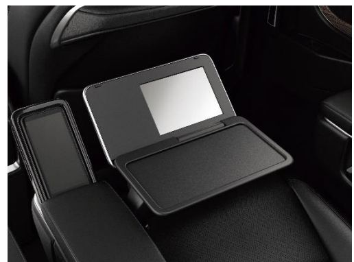
Vanity Mirror With NSG's Anti-fouling Coating Technology
