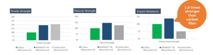
\*Reinforcement fibers added to PA66 at 20%. The data sets are normalized to 100 for E glass composites. The indicated values are measured values and not intended for guarantee use.
