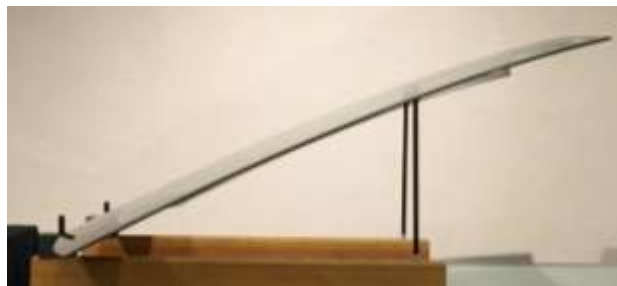
Top: Complex three-dimensional windshield made with advanced press bending method
