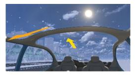
Low-e coatings reduce the amount of outside heat absorbed by the glass and emitted into the vehicle in summer, while in winter they reflect heat from inside the vehicle and reduce the amount of interior heat emitted outside. This reduces the heating and cooling load.
