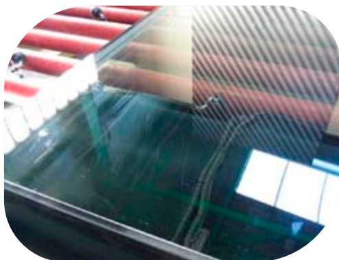
The results of glass cleaning with the use of steel blade – visible surface damages.
