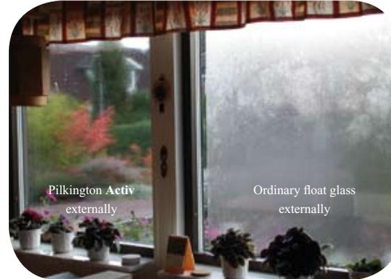
The window to the left has the self cleaning glazing Pilkington **Activ** as the outside pane, and the external view is considerably improved. Furthermore, the condensation disappears much faster from the surface with Pilkington **Activ**, see picture below.
