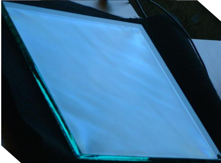
The same 12 inch square of 12 mm tempered glass much more readily shows the quench pattern under the same lighting and viewing conditions when viewed in reflection, with the transmitted image subdued by placing the glass on black velvet.
