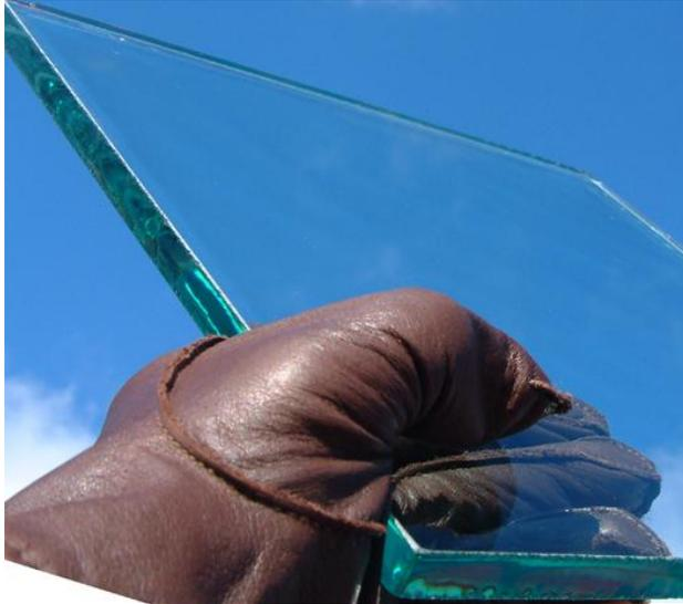
A 12inch square of 12 mm thick tempered glass can show its quench pattern to the naked eye, with no Polaroid filters, when viewed at appropriate angles on a blue sky day.
