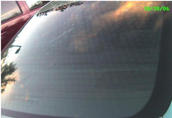
Typical dot quench pattern seen in a tempered Mercedes automotive back window when incoming light is reflected from a blue, or partly cloudy, sky. Notice the sun is not directly shining on the glass.
