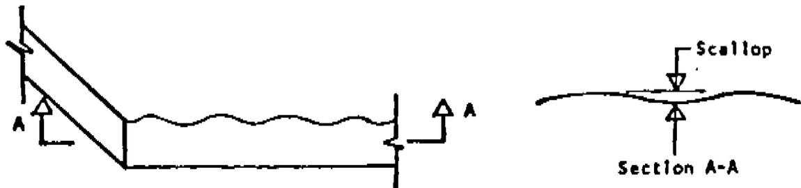
4. **Shell or Flake Chip** - This is a chip at a glass edge, usually smooth, having the appearance of a shell. Flake chips are generally more pronounced as glass thickness increases.
