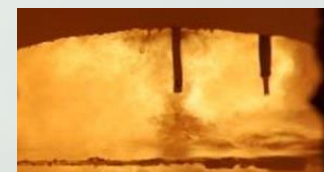
Flame appearance inside the furnace using a fuel blend of 80% natural gas and 20% Hydrogen.
